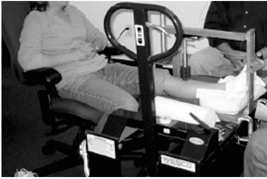
Figure 7. The test setting with a subject sitting on an adjustable chair with her left leg positioned for testing. An adjustable platform (lever and platform) allowed for positioning of the leg at the correct height and angle for all subjects.
